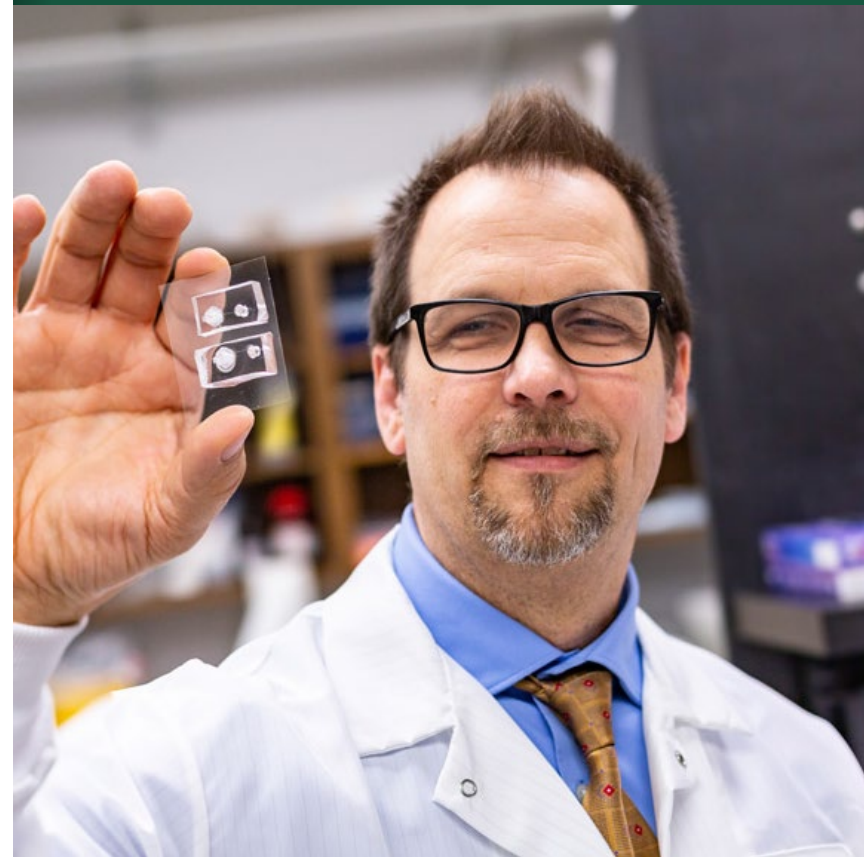
Dr. David Schmidtke displays a microfluidic device used to fabricate tiny strands of collagen called fibrils to advance his team's research on the eye's repair process.
